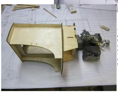
The mount has to be seriously reinforced with internal triangular solid wood stock as the structure is only made up from 4mm ply . The exception is the firewall which is made by laminating two 4mm pieces together.
