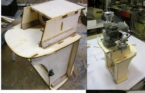
I reinforced the engine mount with 12mm Merranti quad from Bunnings. It's cheap but it's heavy but as I'm not worried about saving weight forward of the C of G it's a good convenient and strong material to use.
