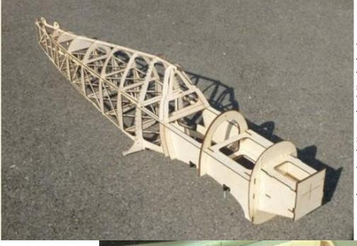
This is a picture of the finished assembled frame from Mick's instructions. The front part of the forward structure is the part that is cut down to suit the motor to be fitted. My motor mount is about half as long as Mick's to suit the Zenoah G62.
