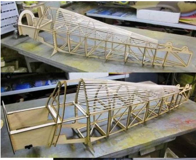
The top section stringers are all done and the radio mast mount and backbone reinforcing for the mast completed.
