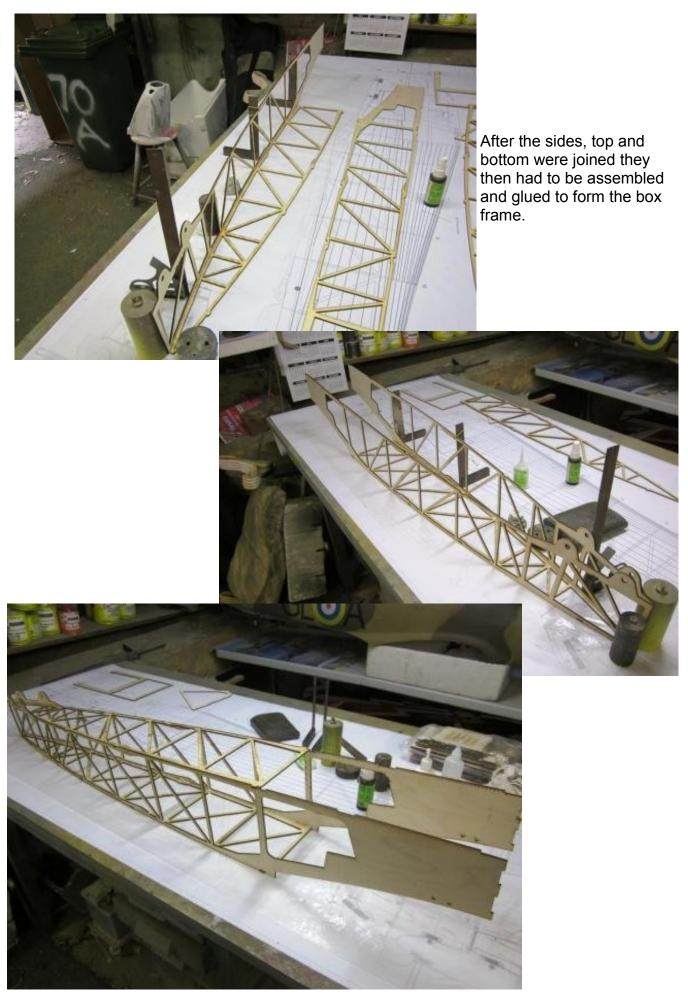
Mick has designed this model to have a fuselage in two parts. The rear part is the basic frame and the front part is a strong plywood structure to mount the motor etc.. The join is forward of mid chord.
