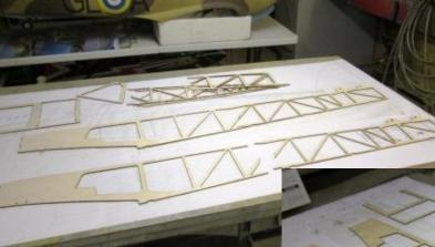
I immediately hit a snag when I found out that CA glue doesn't like the laser cut plywood burnt edges
