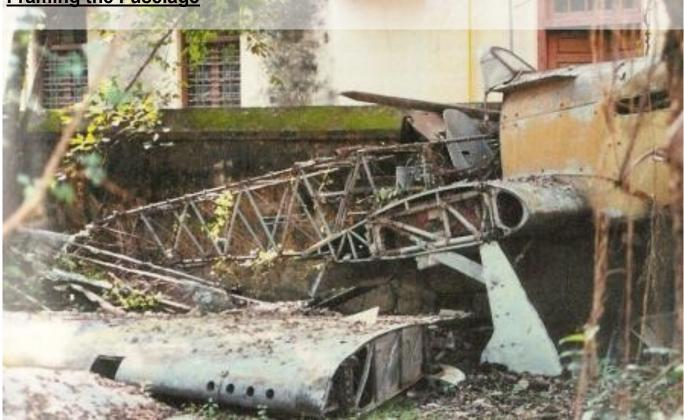
The fuselage on the full size Hurricane is built on a base of a tubular box frame. This frame then has formers and stringers attached to build up the distinctive shape of the Hurricane. The image above is of the Hurricane R4118 that was rescued from India and fully restored. Below is a line drawing of the basic frame structure.
